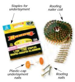
Typical fasteners for a roofing project include staples, roofing nails (both standard and plastic-cap), and coil nails for roofing nailers.
